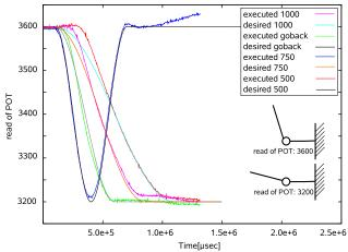
Fig. 4. Different desired and executed trajectories of the android arm after consolidation learning is finished. Time is given in microseconds.
