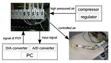
Fig. 3. The setting of the experiment for testing consolidation: An android arm is actuated by air pressure coming from a compressor.
