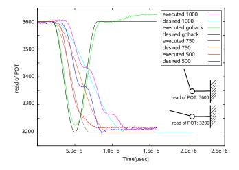
Fig. 5. Different desired and executed trajectories of the android arm after Feedback-error learning with static network of 20 hidden neurons.
