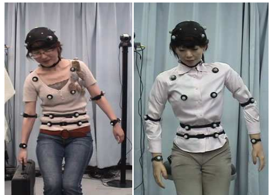
Fig.4 The performer's and mapped postures (having a heavy baggage, \bar{\delta} = 37.5\text{mm} , \sigma_s = 13.2\text{mm} ).
